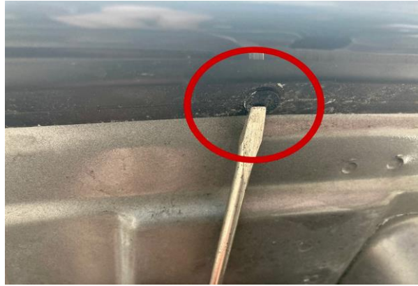
Align bonnet guard to show the four plastic clips to remove
