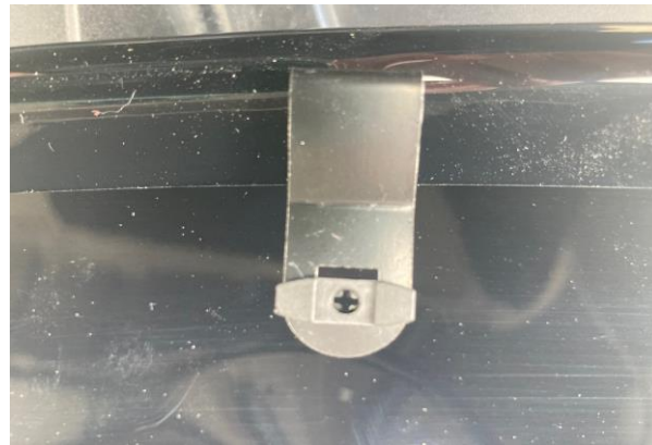
Insert four plastic plugs through the square hole into existing hole in bonnet
