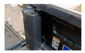
Remove the rear tie down points, Attach the rear bracket, fit together with the original tie down points. Do not tighten
