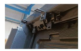
Lift Roller top into place and pull back ensuring clearence with the tailgate.
