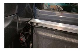
Remove plastic side covers. Fix the bulkhead bar using the 2 bolts, fitted into the 2 threaded holes
