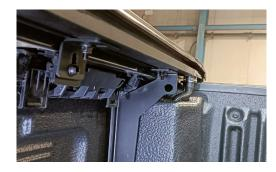
Line up T-bolts with the side brackets, fit and tighten the M6 nuts. Then tighten all side arm bolts.
