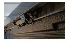
Remove the two bolts from the Wildtrak side arms and re-fit, together with the right anlge brackets
