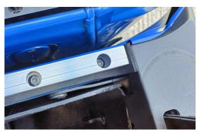
Step 5: Remove pictured blocks from the feet of the Roll bar (leave the rubber foot in place).
