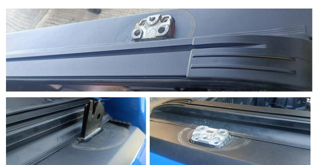
Step 7: Use the bolts removed to spread the roll bar wider (see image below) and bolt into position.
