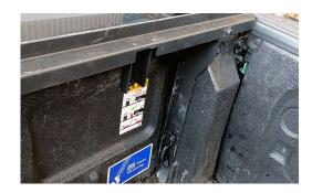
Remove the rear tie down points and fit the bracket - Align side arm and bolt to bulkhead and rear bracket (allowing for the tailgate to close)
