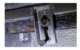
Set bolts in to bottom holes to stop the bracket from twisting
