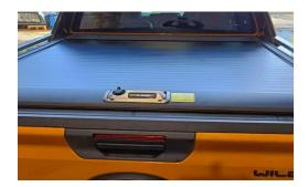
Pull the Roller top back and ensure clearence with the tailgate. Then tighten all side arms
