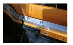
Fix the bulkhead bar using the 4 bolts, fitted into the 4 threaded holes
