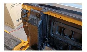
Attach the rear bracket, fit together with the original tie down points. Do not tighten
