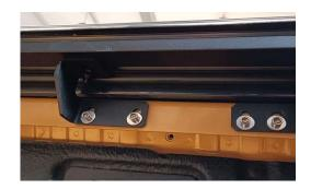
Line up the T-bolts with the side brackets, fit and tighten M6 nut
