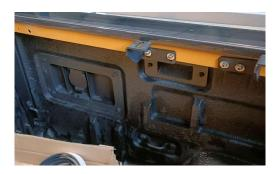
Attach side brackets, do not tighten. Lift Roller top into place.
