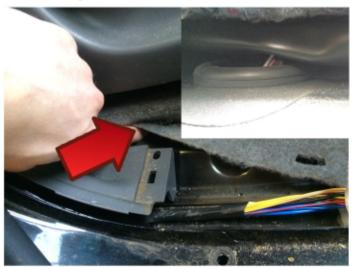
4) Lift the carpet underneath the drivers door. This will reveal a rubber grommet using this grommet, pass the '2-wire' leg through the hole to the underneath of the vehicle and fill with silicon sealant. Attach the wiring loom to the chassis (as shown above) and connect the wires to the canopy.
