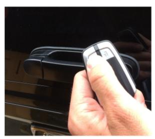
Check that the hardtop locks and unlocks using the vehicle's remote.
