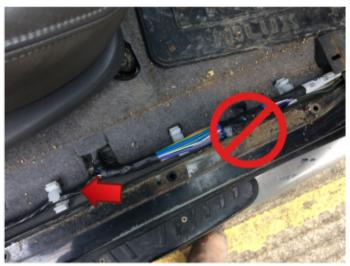
2) This will reveal the wiring. Expose the wires as indicated by the arrow above.
